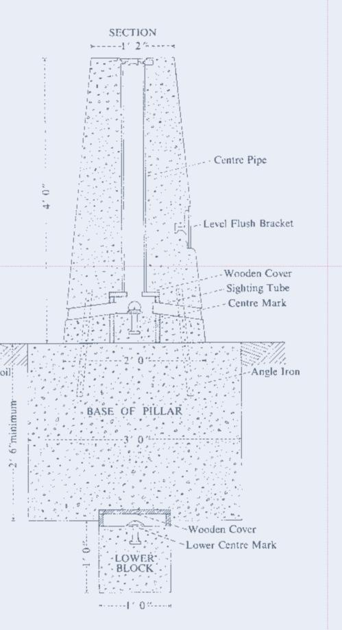
A trig point, or more correctly, a standard concrete triangulation pillar, used to mark the primary stations of the Ordnance Survey's retriangulation of Great Britain 1935-62 - a project that sought to improve the accuracy of the country's maps. Trig points have now been replaced by global satellite navigation systems. Although redundant, they still remain powerful objects in the landscape.
